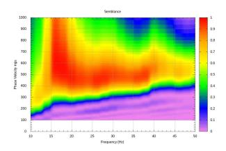
Figure 35: BVAS: SH body-wave semblance results for down-hole data.
