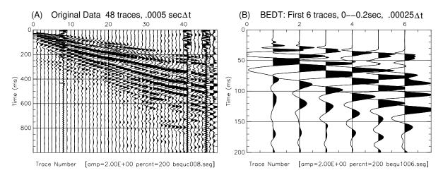
Figure 73: BEDT: (A) Original data, 48 traces, 0-1 seconds, .0005 second sample interval. (B) Edited to only first 6 traces, 0-0.2 seconds, interpolated to .00025 second sample interval.
