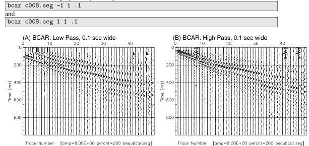
Figure 107: BCAR: (A) low-pass filter, trace equalized with BEQU 12.0.9 (B) high-pass filter by subtracting low-pass from original data, also trace equalized. Input data are same as in Figure 106A.
