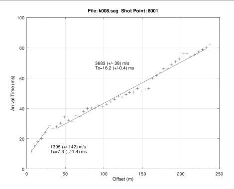
Figure 16: OCTAVE REFPLOT: Plots first break picks which have been added to headers with BPIC. Then use mouse to pick line segment (start,end), followed by a mouse click to plot refractor apparent velocity result. See section 8.5.6, estimating a cross-over distance for program BREF.
