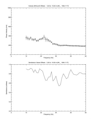
Figure 19: BVAX: Phase velocity semblance display file, bvax.ps. These are the autopicks from figure 18.
