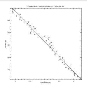
Figure 30: BFIT: Straight line fit yields interval velocity by least squares. Title has the value of the velocity, 479  $\pm 10$  m/s.
