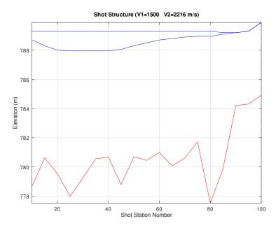
Figure 49: OCTAVE DELAYTMR: Structure assuming an overburden velocity of 1500 m/s. River water surface and bottom of river bottom in blue. Refractor structure in red.
