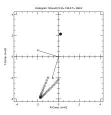
Figure 65: BHOD: plot produced showing PCA results for a geophone at about 19.39 meters depth. File bhod.lst: (00010 196.8 286.8) = (seq. R-azi, T-azi)
