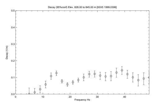
Figure 36: BAMP: SH body-wave amplitude decay for down-hole data same as seen in Figure 34 velocity dispersion. Corrected for beam spreading, a viscous, Kelvin-Voigt material, the decay should increase with frequency (Michaels, 1998).
