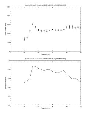
Figure 34: BVAS: SH body-wave dispersion and semblance results for down-hole data. These are the automated picks for maximum semblance as seen in Figure 35. Viscous, Kelvin-Voit behavior is an increase in velocity with frequency (Michaels, 1998).
