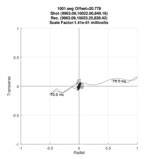
Figure 12: OCTAVE HODOPLOT: Plotting particle motion on the down-hole horizontal R- and T- components which are channels in the same \*.seg file. If components are in different files, use HODO2PLOT program instead (see 6.0.10).
