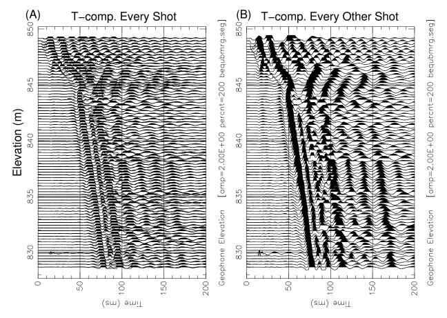
Figure 72: BMRG: A)is plot of all shot efforts (166 traces) and B) is plot of only very other shot (83 traces). NOTE: data are not rotated to a standard orientation, azimuth of T-component drifts up the hole.
