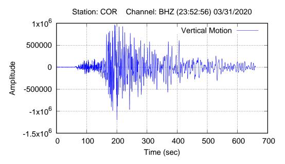
Figure 3: Image produced from Gnuplot and the output \*.gp file from mseed2seg. The title gives the Station, Channel, initial time of day for zero time on the plot, and the date of the earthquake.
