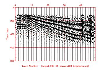
Figure 76: BWIN: Data zeroed outside of the tapered window.
