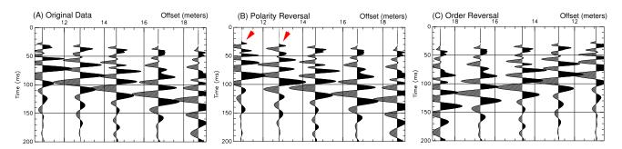
Figure 78: BREV: (A) original data, (B) reverse polarity first 2 channels, (C) reverse channel order. Data plotted by offset.
