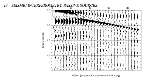
Figure 117: GENBIMG: Output file STAK.seg is the sum of the BIMGxxxx.seg files for the different time windows. Note that the time scale is 0 to 2.0 seconds with zero lag at 0 seconds. **Mix was set to zero**.
