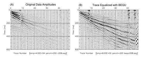
Figure 82: BEQU: (A) original scaling of data, (B) trace equalized with L2 norm. The scale factors for plotting are 40000 for (A) and 8 for (B).
