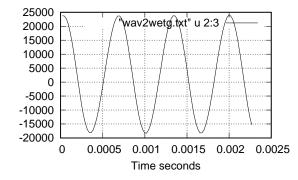
Figure 2: Blowup of the carrier frequency (about 1500 Hz), first 100 samples of Figure 1.
