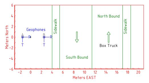
Figure 122: GENBAZI: Layout of geophones that recorded signals from a box truck traveling north.
