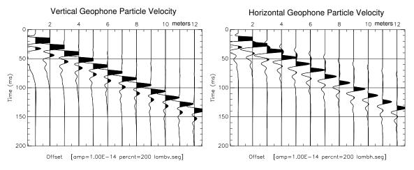
Figure 53: LAMB: Geophone (10 Hz, 0.7 damping) response, itype = 6.
