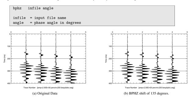
Figure 98: Comparison of original and shifted data.
