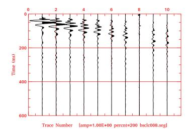
Figure 83: BSCL: Scale all traces by the maximum absolute value (MAV) found in the first 5 traces.
