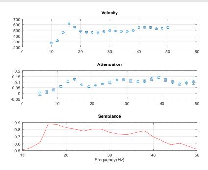
Figure 37: CAINV3: First display. Use mouse to pick frequency limits for analysis, low and then high. After running **cainv3**, you may wish to make nice plots. For this, there is program **caplot3** (8.3.8).
