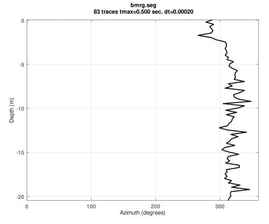
Figure 11: OCTAVE SEISAZI: Plots a horizontal component azimuth from the headers of an \*.seg file. Here, the plot is of the T-component from a down-hole survey. Phone orientation was determined using program BHOD.
