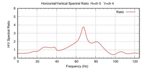
Figure 128: HVSR: The ratio between horizontal and vertical components (H/V) is computed from the spectra shown in Figure 127. Note that below about 20 Hz, the vertical motion dominates.
