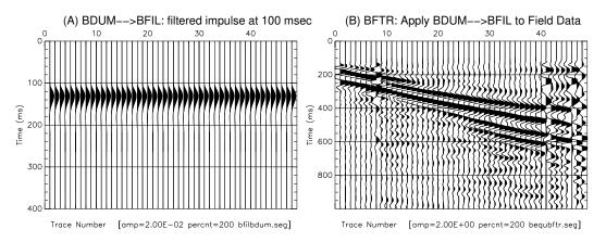
Figure 110: (A) BDUM–>BFIL: Filtered file of impulses. (B) BFTR: Filter field data with filtered impulse file. Input data **c008.seg** are same as in Figure 106A.
