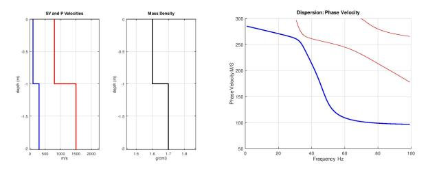
Figure 56: DISPER: The model and phase velocity plots. The model.m plot shows P-wave (red), S-wave (blue) velocity, and density (black). This is a layer over a half-space model. On the right is the phase.m generated plot showing the fundamental mode (blue) and two higher modes (red). The model (soil profile) was generated in gendis (9.2.5)
