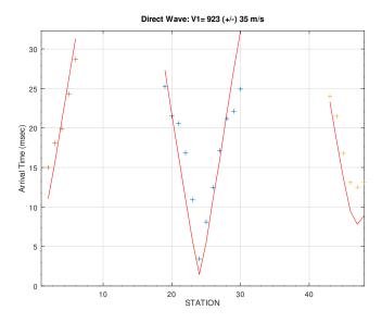
Figure 45: BREF: Output plot.ps for direct wave analysis. Title shows the least squares solution for the overburden velocity,  $923 \pm 35m/s$ . Range of offsets 0 -> 30 m.
