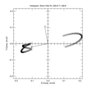
Figure 67: BHOD: plot produced showing PCA results for a geophone at about 20 meters depth.
