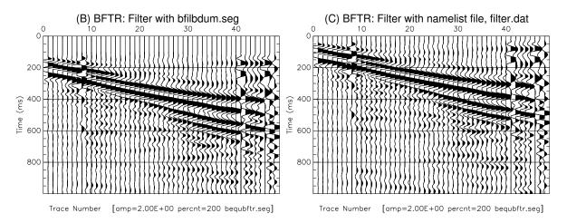
Figure 111: (B) BFTR: same as in Figure 110B. (C) BFTR: Filter field data with namelist file, **filter.dat**. Input data **c008.seg** are same as in Figure 106A. Note the different time delay due to placing an impulse at 100 ms (Figure 110A) in the filtered BDUM, compared to the start time in the TRAPLT approach (.09 sec).
