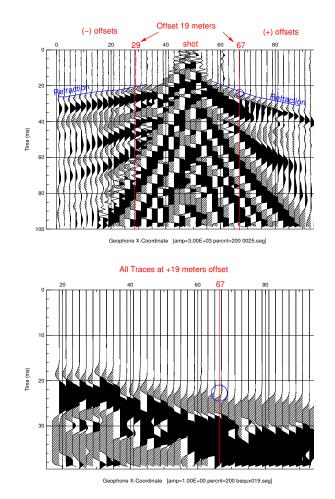
Figure 77: BXOF: A shot gather at station 25 shows a first arrival on the refraction is clear at an offset of +19 meters. Below is a collection of +19 offset traces. The overburden appears to thicken from left to right. The first arrival also seems to exhibit a measure of high frequency loss, possibly due to inelastic attenuation. Data provided by Yilmaz *et al.* (2022).
