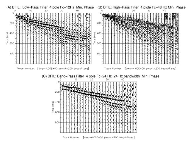
Figure 108: BFIL: Input data are same as in Figure 106A.
