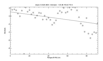
Figure 84: BGAR: Broadband scale by spherical divergence and exponential decay. Range from 6 to 100 meters.
