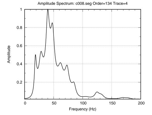
Figure 10: OCTAVE YULE WALKER: Octave program which computes the ALL POLE spectrum. Input can be either a seismic trace data or an autocorrelation of trace data (either must be in BSEGY format, \*.seg file). Compare to Figure 9 FFT plot. See BXCR 12.0.16 for how to create an autocorrelation as input.
