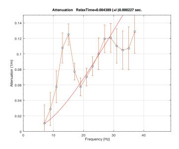
Figure 39: CAPLOT3: Plot of decay, measure and calculated (solid line) only over frequency range used in cainv3 (8.3.7). Weighting by reciprocal of standard deviations. Relaxation time about 4 msec. Relaxation time is  $T_r = \frac{C_2}{C_1}$ .
