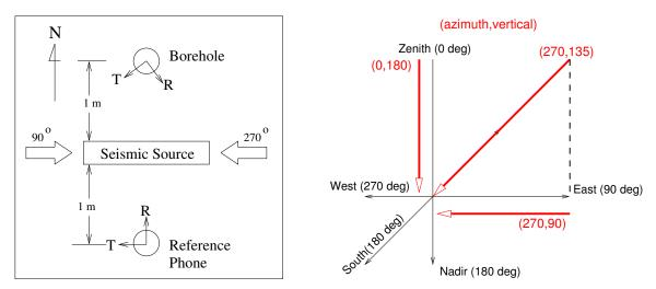
Figure 105: The author's orientations and notation for down-hole surveys. Note that the reference and bore-hole phones are wired differently (in terms of R- and T-component wiring).
