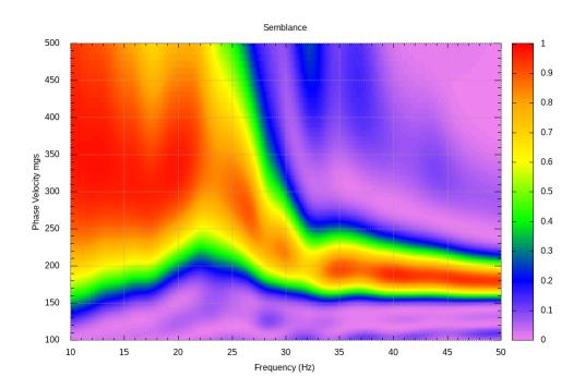
Figure 18: BVAX: Phase velocity semblance display file, clrplot.png. For details on semblance, see Sheriff (1991). Semblance provides a measure of the degree to which the data were aligned at a trial velocity. Offset range was limited:  $5 \rightarrow 19$  meters.
