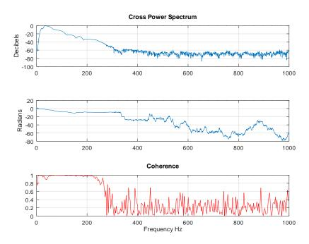
Figure 23: SASW: Cross spectrum amplitude and coherence reveal what range of frequencies provides useful dispersion information.
