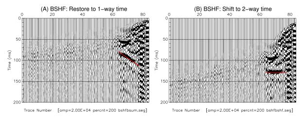
Figure 104: BSHF: (A) Restore to 1-way time, down going removed (see figure 103 B) (B) BSHF: Shifting data in (A) to 2-way time. Reflections should be horizontal.
