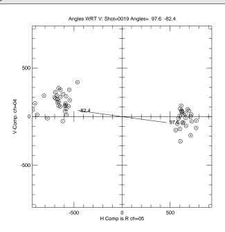
Figure 125: BZRT: Motion in the vertical plane as truck passes the geophones in the 8.0 to 9.0 time interval. Note that the polarization ellipse major axis is essentially horizontal. One does not know for sure what type of wave motion has been captured. It is possible that we are looking at more than one mode of Rayleigh wave.
