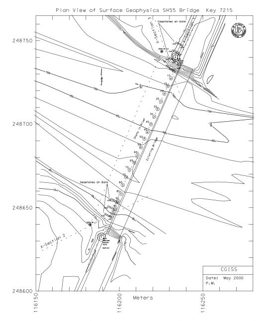
Figure 48: OCTAVE DELAYTMR: Reciprocal shooting across a river. Airgun source deployed at stations across bridge (Michaels, 2001a).
