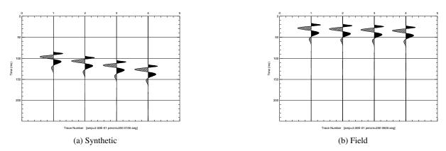
Figure 96: Two shot gathers to compare with no overlap.  $STD(\Phi_k) = 0$ ,  $\overline{\Phi} = 90^\circ$ , and OBF = 80.
