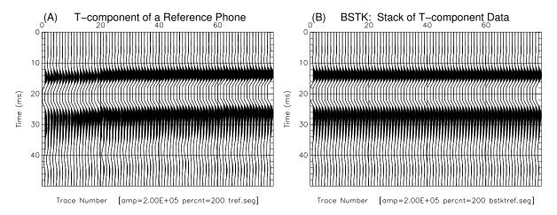
Figure 91: BSTK: (A) Original data T-component data (B) Stack of the T-component data (all traces replicas of the stack result). An application might be creating a target for wavelet processing (BSHP 12.2.1).
