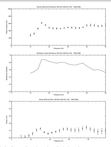
Figure 8: CAPLOT: Display S-wave dispersion and amplitude decay from program outputs of BVAS and BAMP programs.
