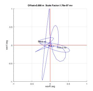
Figure 60: Hodogram for offset 5 meters. Requires bsegin.m, segyinfo.m, and hodo2plot.m in directory with wavV.seg and wavR.seg files (see 6.0.10).
