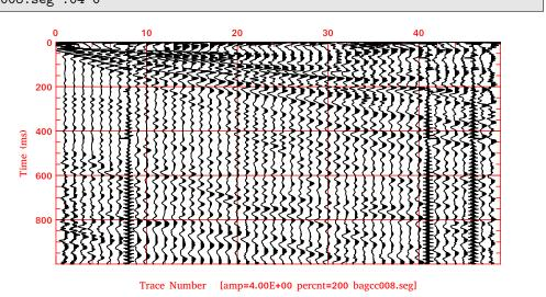
Figure 89: BAGC: Single pole AGC envelope .04 seconds.
