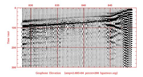
Figure 87: BGAZ: Broadband scale by spherical divergence and exponential decay. Specified 1.43 dB/m for inelastic decay. Elevations are down the bore-hole.
