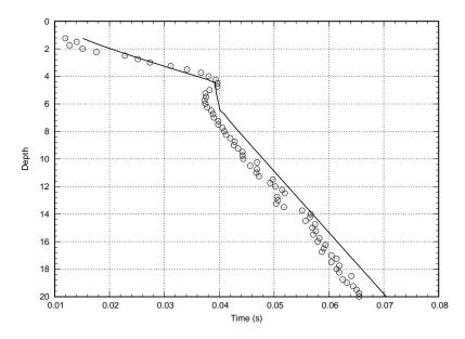
Figure 33: BVSP: Solution is a first layer, 4.5 meter thick Vs=114.3 m/s, second layer 2.0 meter thick, Vs=459.7 m/s, on top of a half-space with Vs=395.1 m/s.
