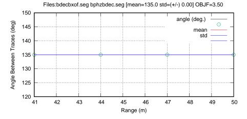
Figure 99: BOBF analysis of data (figure 98(a)) and after BPHZ  $135^{\circ}$  phase shift (figure 98(b)). Note that the standard deviation on the angle is zero, but the maximum amplitude moves to a different sample after the shift, resulting in an objective function value of OBF=3.50 (see equation 20)
