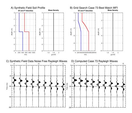
Figure 28: The soil profiles and computed shot gathers for the synthetic field data (A) and the best fit (B) (grid point labled min on figure 27).
