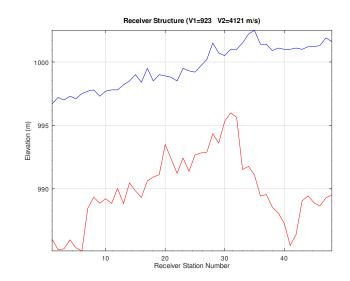
Figure 46: OCTAVE DELAYTM: Structure solution for shots k008 and k009. Ground surface in blue, top of bedrock in red. Soil velocity 923 m/s between blue and red. Bedrock velocity 4121 m/s.
