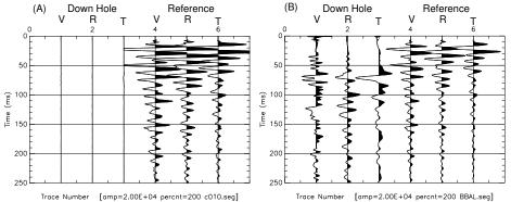
Figure 90: BBAL: (A) Original data (down-hole barely visible) (B) data after splitting the data into two files, running BBAL, then combining into a second file. This figure was created using the XFIG program and the \*.fig output type in BPLT 6.0.2
