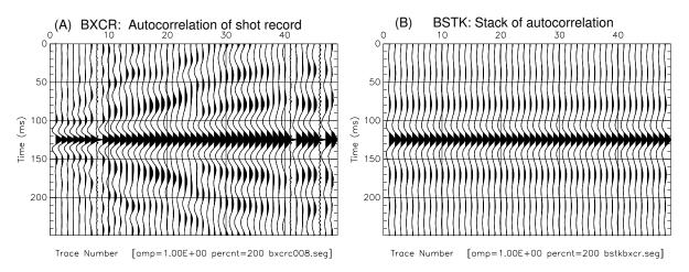
Figure 92: BXCR: (A) Auto correlation of data shown in Figure 82 (B) Stack of the auto correlation (all traces replicas of the stack result).
