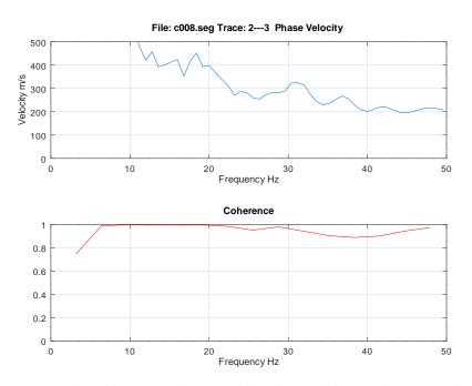
Figure 24: SASW: Dispersion computation over limited range of frequencies selected in the GUI.
