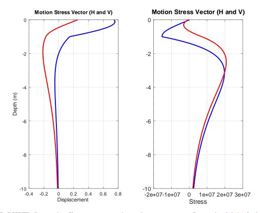
Figure 57: DISPER: Re-running **disper** to compute the motion stress vectors. See section 9.2.6.1 for how to edit **disper.d**. The file, mat2.m created this plot. Blue is horizontal, Red is vertical.
