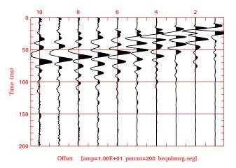
Figure 63: GENWAW: Example data from a small hammer source, trace equalized with BEQU 12.0.9.
