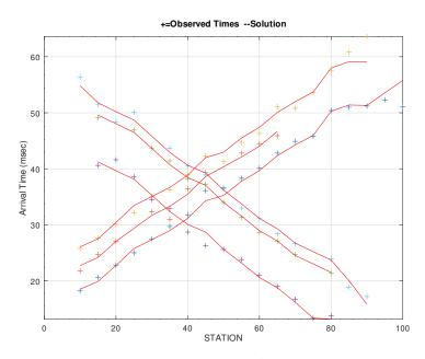
Figure 50: OCTAVE DELAYTMR: Observed arrival times and fit assuming an overburden velocity of 1500 m/s.
