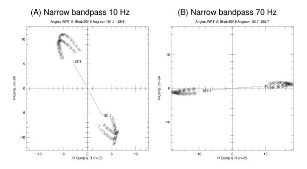
Figure 129: BZRT: Hodograms of narrow band-pass filtered data. Time interval 8.4 to 8.6 seconds. Zero-phase 18 pole filters (bandwidth 0.4 hz) with center frequencies of 10 and 70 Hz. Compare these plots with the HVSR ratio in figure 128.
