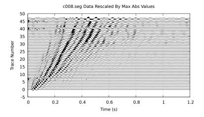
Figure 7: QPLT: Quality control plot showing traces, **each scaled by the maximum value in the trace**. Output includes X11 and qgraph.gp (GNUPLOT). Edit qgraph.gp to change terminal type (ie. postscript) and run qgraph.gp with gnuplot.
