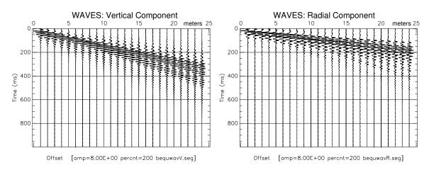
Figure 59: WAVES: Synthetic seismograms for Vertical (wavV.seg) and horizontal (wavR.seg) motion.
