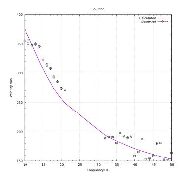
Figure 22: invR1: The code also generates a GNUPLOT file, disperv.gp, which shows the final solution when run with the gnuplot program.
