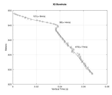
Figure 32: VFITW –>VPLOT: Plot of vertical time vs. elevation, and interval velocities. Axes and placement of velocity labels by mouse.
