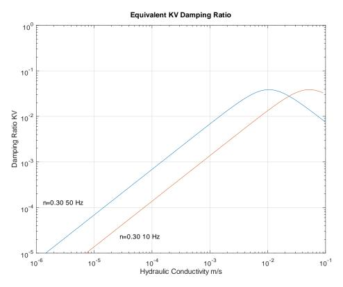
Figure 40: kdKVMBscan.m: Plots Kelvin-Voigt damping ratio vs. hydraulic conductivity for user provided porosity and frquency of shaking. Here, porosity is 30% and frequencies are 10 and 50 Hz. Left of the peak is coupled motion (small pores, fluid largely moves with frame). Right of the peak is uncoupled motion (large pores).
