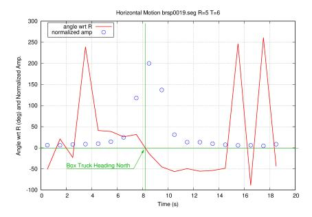
Figure 124: GENBAZI: Result of running **gobazi** bash script generated by the **genbazi** command above. Note that the angle (plotted in red) crosses zero at about 8.5 seconds, and this agrees well with the normalized amplitude on the horizontal components. Assuming a geophone to truck distance of 12 meters, the slope of the angle with time suggests a vehicle speed of about 18 mph.
