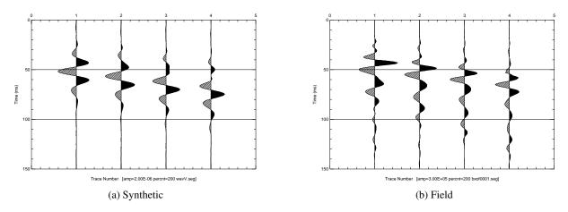
Figure 94: Two shot gathers to compare,  $\overline{\Phi} = 43.3^{\circ}$ , and  $STD(\Phi) = 4.12^{\circ}$ .
