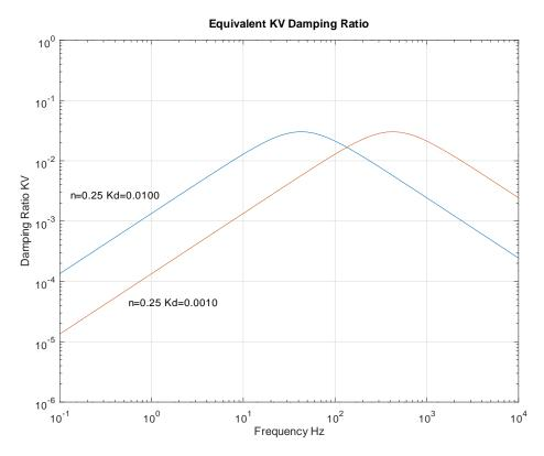
Figure 41: fqKVMBscan.m: Plots Kelvin-Voigt damping ratio vs. frequency fo user defined porosity and hydraulic conductivities. Here, porosity set at 0.25, two different cases of hydraulic conductivity  $K_d = .01 \ K_d = .001 \ m/s$ .
