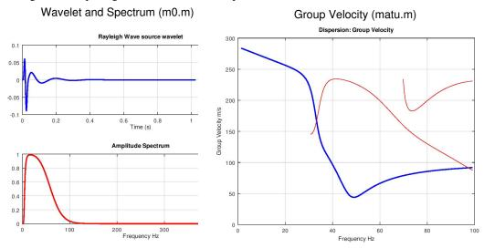
Figure 58: WAVES: Wavelet on left, group velocity dispersion on right. No significance to curve colors except that in the dispersion plot, the fundamental is Blue and higher modes are in Red. Soil representation is layer over half-space as shown in 9.2.5.1 and Figure 56 above.
