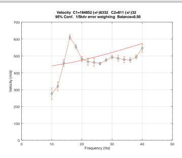
Figure 38: CAPLOT3: Plot of velocity dispersion, measure and calculated (solid line) only over frequency range used in cainv3 (8.3.7). Weighting by reciprocal of standard deviations.
