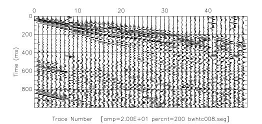
Figure 112: BWHT: 0.4 second AGC window, 50 Hz center, 80 Hz bandwidth, 10 Hz rolloff. Input data **c008.seg** are same as in Figure 106A.
