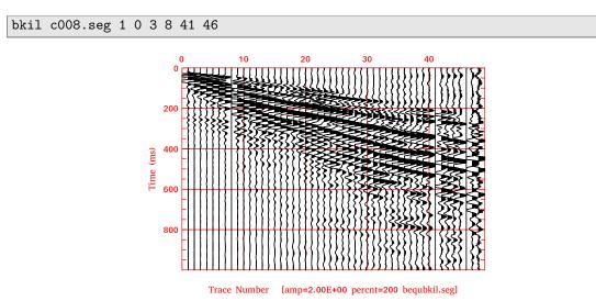
Figure 74: BKIL: Zero noisy traces 8, 41, 46 of data shown in Figure 73 (A).
