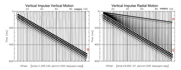
Figure 54: BNFD: Computing all fields (S-wave, P-wave, Near-field) The geometry is taken from a template file, c008.seg, and spans offsets from 7 to 100 meters. As offset increases, the far field P- and S-wave motion waxes as the near field wanes.
