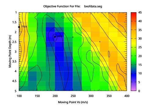
Figure 29: Contour plot of the objective function for the **BWFI** example run. The soil profile and waveforms of the objective function minimum are shown in Figure 28) (B) and (D).
