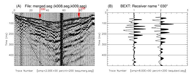
Figure 75: BEXT: Extracted traces from receiver location "030". In the merged file (A) red arrows show receiver "030" and these are replotted in (B). Note the receiver name is 4 characters, "blank,zero,three,zero".
