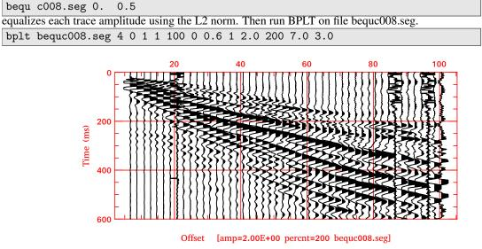
Figure 5: Trace equalized version of Figure 4
