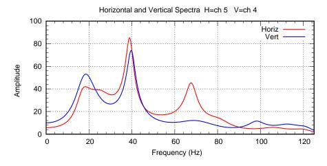
Figure 127: HVSR: We focus on the time interval from 8.0 to 9.0 seconds when the truck passes the geophones. The data are time series recorded from phone B (see figure 122). The instrument analog low pass filter has a cut-off frequency of 100 Hz.
