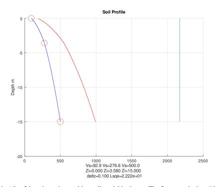
Figure 20: invR1: After 5 iterations, the resulting soil model is shown. The S-wave velocity with inverted control points is shown as the Blue curve (m/s). The Red curve is the P-wave velocity, and at the far right is the constant density  $(kg/m^3)$
