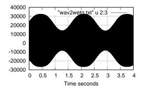
Figure 1: Example of an AM modulated carrier sampled at 44100 samples/second.
