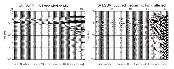
Figure 103: BMED: (A) median mix of the direct wave (see figure 102 B) (B) BSUM: direct down-going wave estimate subtracted from total wave field.
