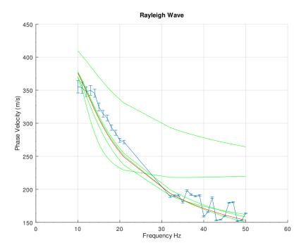
Figure 21: invR1: Progress of the inversion. The initial model dispersion is the fastest green curve. The green curve is the dispersion after 5 iterations. Data from bvax.his is in blue.
