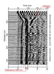
Figure 31: BVEL: Data flattened on 500 m/s (direct wave in bedrock). Overburden is slower (about 100 m/s). Reflection off top of bedrock shown.
