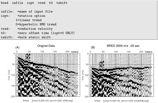
Figure 17: (A) Plot of a shot gather, (B) BRED: linear trend, 3000 m/s reduction velocity, .05 seconds offset. See section 8.5.0.1 for an example of picking data with BRED.
