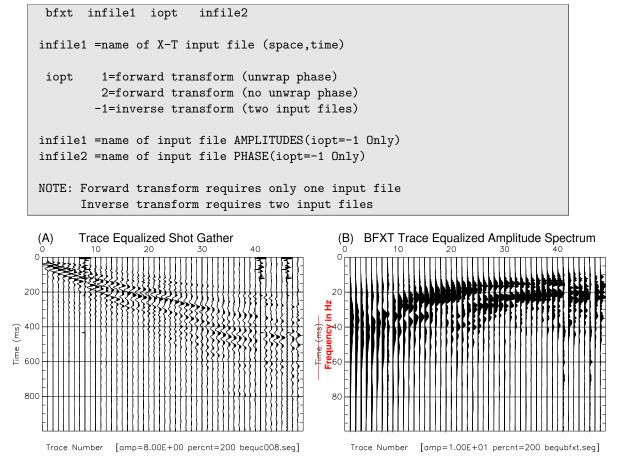
Figure 106: BFXT: (A) trace equalized shot gather using BEQU 12.0.9 (B) the amplitude spectrum after equalization with BEQU. Not shown is the phase transform.
