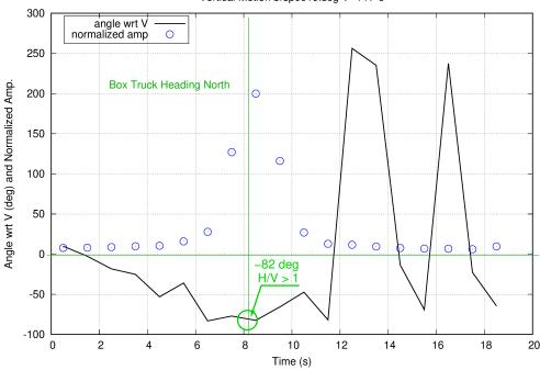
Figure 126: GENBZRT: As the truck passes the geophones, recorded waves are stronger on the horizontal rather than the vertical component. To explore this in greater detail, consider running program **HVSR**.
